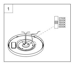
Step 1: Selecting the correlated Color Temperature (CCT). Before installation, select your preferred CCT by moving the switch to either 2700K, 3000K, 3500K, 4000K, or 5000K
