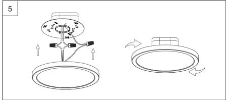
Step 5: Attaching the LED fixture to the Junction Box. Push the LED fixture into the mounting plate and make sure the LED fixture is fully secured before releasing.
