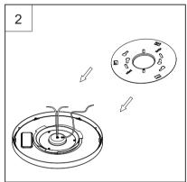
Step 2: Preparing the Mounting Plate. Choose the mounting plate holes compatible with your junction box.
