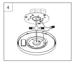
Step 4: Making the Wiring Connections. Using the included wire nuts (BB), connect the black wire to the hot supply wire, Connect the ground wire (green wire) to the ground wire, and connect the white wire to the supply neutral wire.
