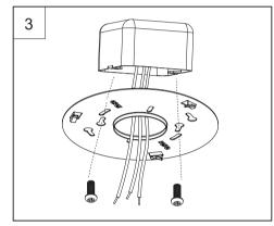
Step 3: Installing the Mounting Plate. Align the appropriate holes in the mounting plate with the holes in the junction box. Using the screws, attach the mounting plate to the junction box. Tighten the screws until the mounting plate is flush with the ceiling.
